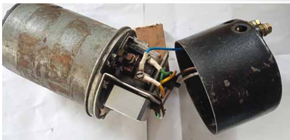
Fitting the DVR2 inside the dynamo end cover
