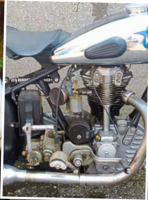
Over the decades that the 251 OSL was in production, its gearchange was swapped from hand to foot operation. Note the distance between the footrest and the gear pedal
