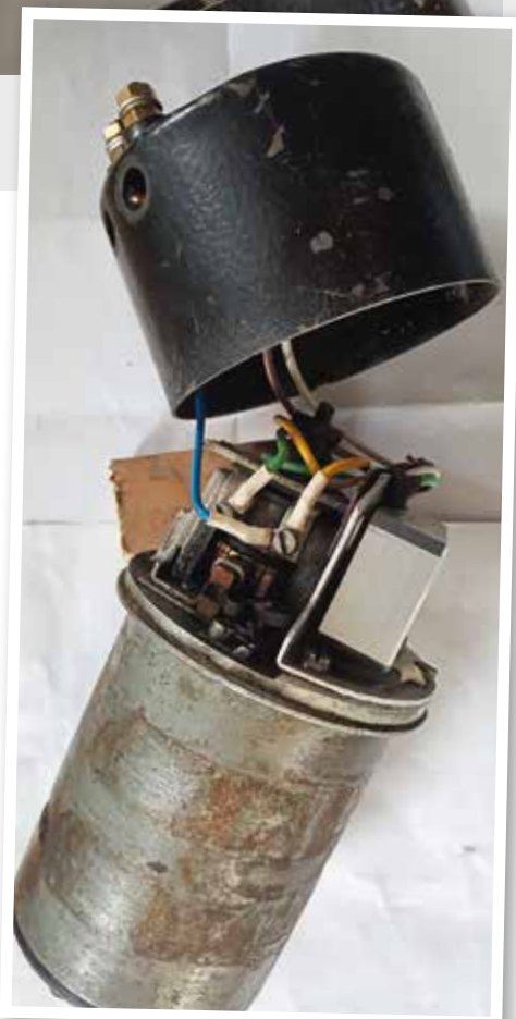
Another voltage regulator, hooked up temporarily to see what would happen with the engine running
