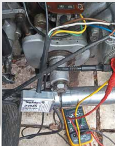
Another voltage regulator, hooked up temporarily to see what would happen with the engine running
