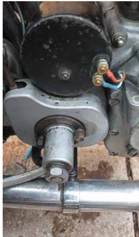
The dynamo with its cover, back on the bike. A rubber boot was added later over the terminals to protect against the weather
