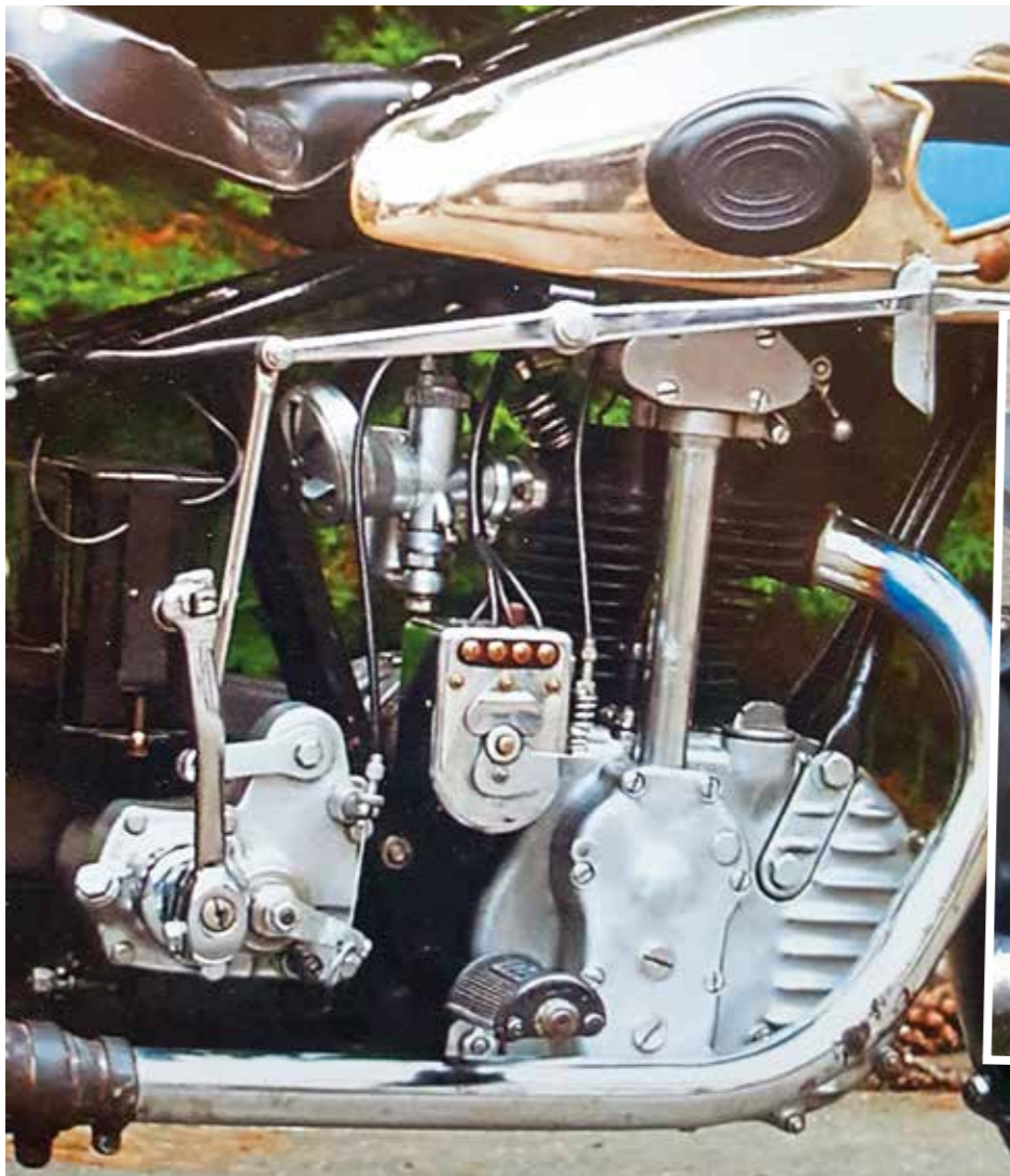
The dynamo with its cover, back on the bike. A rubber boot was added later over the terminals to protect against the weather
