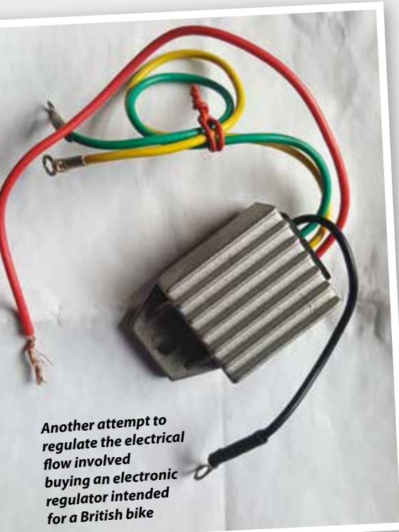
Another voltage regulator, hooked up temporarily to see what would happen with the engine running
