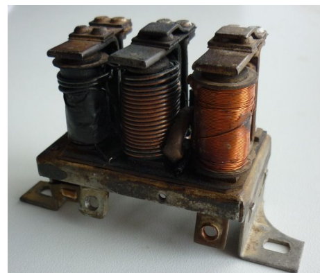
Burnt-out Siba controller
