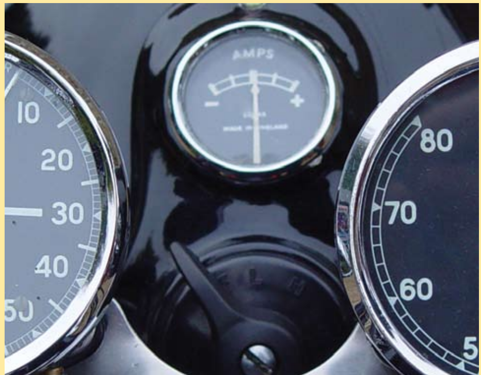
It's easy to get distracted by speedo and tach; the ammeter lets you know about the health of your charging system, and deserves a little attention
