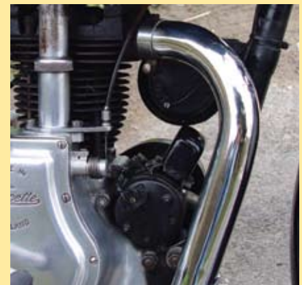
Velocette riders will be familiar with the Miller charging circuit. In this example, the voltage regulator is mounted above the dynamo
